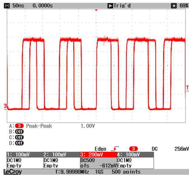
Figure 21: The TIMEPULSE2 signal of the U-Blox LEA-6T receiver configured at 10 MHz is subjected to considerable jitter.
